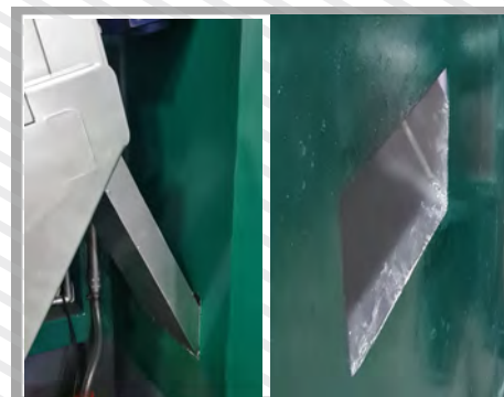
Sludge Cake Discharge Internal / External
