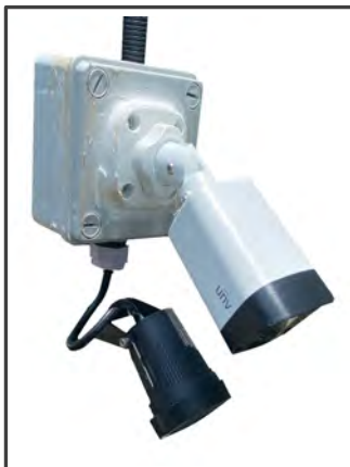
CCTV System complete with LED light
