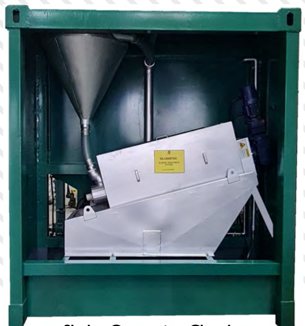
Sludge Conversion Chamber
