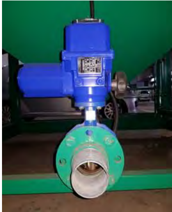
Automatic Sludge Discharge
