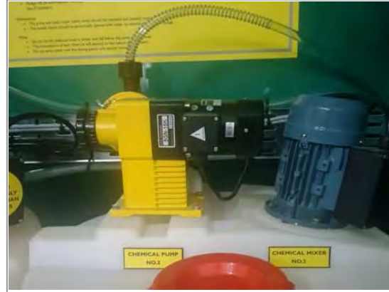
Automatic Chemical Mixing & Dosing System
