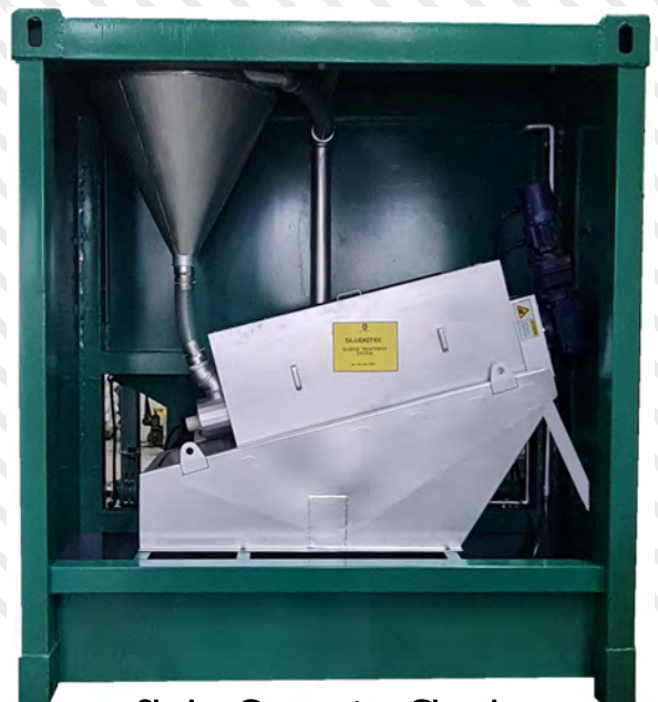
Sludge Conversion Chamber
