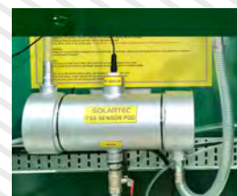
Built-in Chemical Dosing Chamber complete with TSS Sensor Pod - no need for separate TSS Measuring Tank
