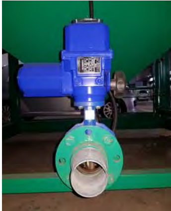
Automatic Sludge Discharge
