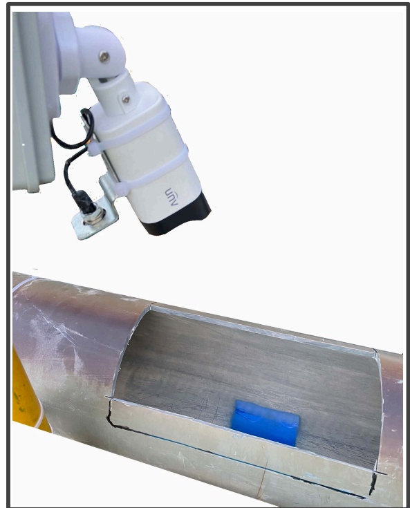
CCTV System complete with LED light and blue marker in Discharge Pipe
